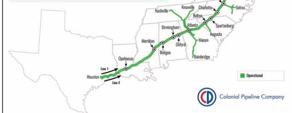
The Colonial Pipeline system is about 5,500 miles long, beginning in Houston, Texas, running northeastward across 13 states, and ending in Linden, New Jersey.
